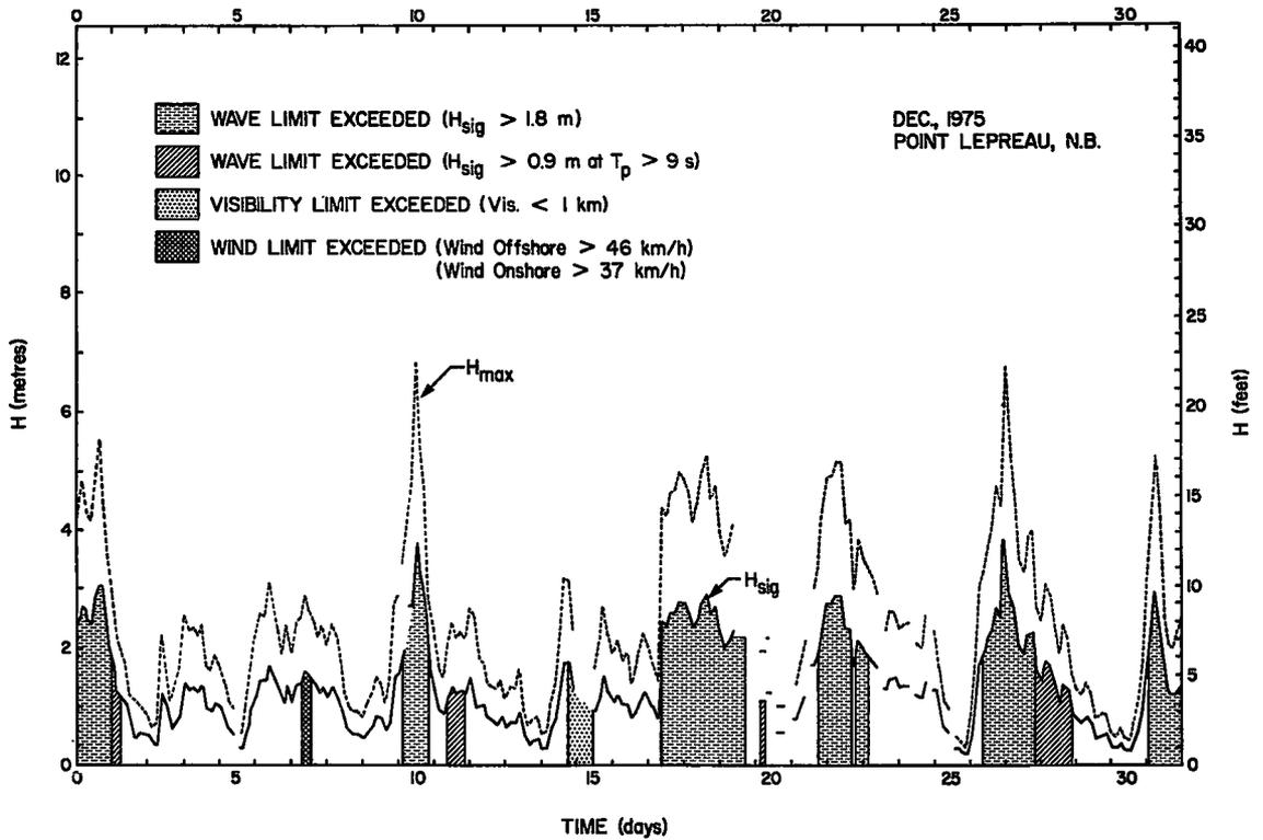
Figure 7. December 1975 wave record at Point Lepreau showing periods of down time.
