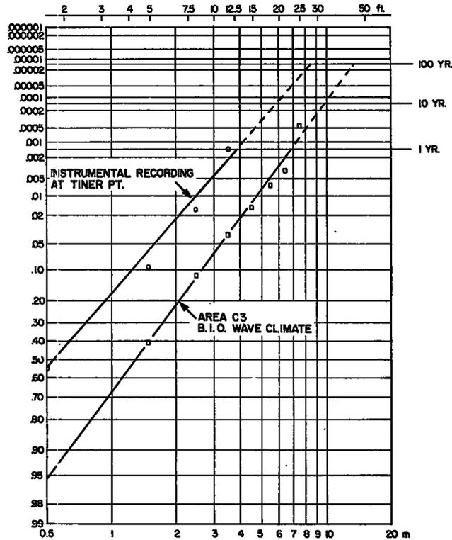
Figure 4. Significant wave height distribution at Tiner Pt. and entrance to Bay of Fundy (Area C3).
